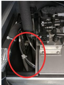
7. Insert the drain tube (located at the back of the appliance).
